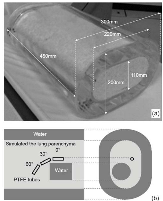
**Figure 1.** An airway phantom placed on the computed tomography (CT) scanner table. The (a) phantom sizes and (b) components of the phantom are shown.
