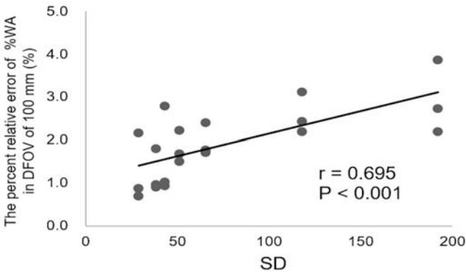
**Figure 4.** The correlation between the SD and the percent relative error of the %WA using a DFOV of 100 mm.
