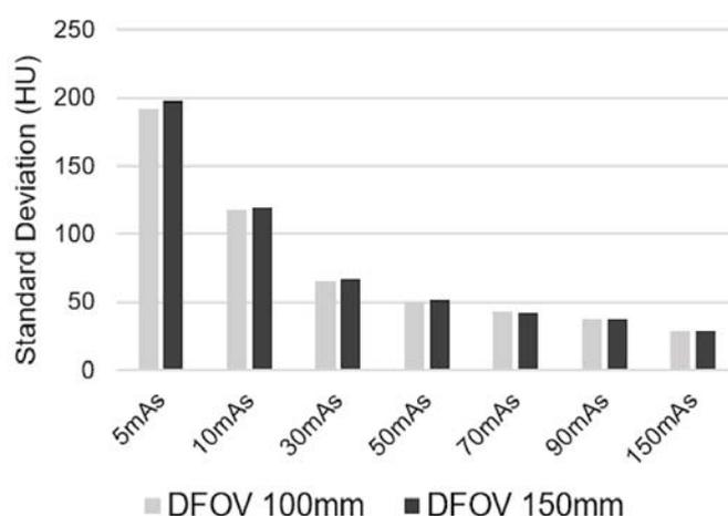
**Figure 3.** Noise measurements, defined as the standard deviation of computed tomography (CT) values in a water phantom, of CT images obtained at 5, 10, 30, 50, 70, 90, and 150 mA. The measurements were performed using a display field of view (DFOV) of 100 and 150 mm.
