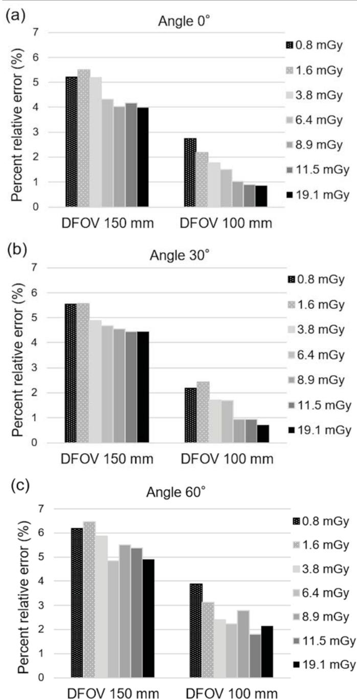
**Figure 6.** The percent relative error of the wall area ratio using a display field of view (DFOV) of 100 and 150 mm for different volume computed tomography dose indexes obtained at tube angles of (a) 0° (b) 30°, and (c) 60°.
