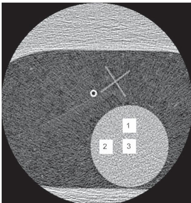
**Figure 2.** Cross-sectional images of 3 ROI placements. Noise measurement was considered the standard deviation of computed tomography values in a water phantom, and was measured in 3 square ROIs (1 central and 2 peripheral).
